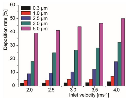
**Figure 5. Variation of deposition rates at different inlet velocity**
