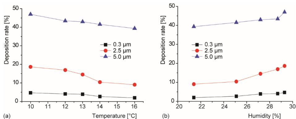
**Figure 6.** Variation of deposition rates at an inlet velocity of 2.0 m/s; (a) deposition rates vary with temperature and (b) deposition rates vary with humidity
