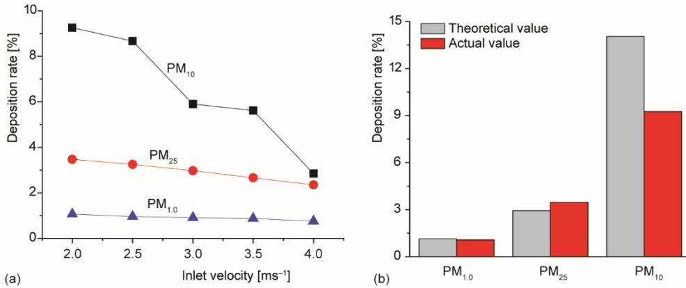
**Figure 3. Deposition rates of PM; (a) deposition rates vary with inlet velocity and (b) differences of deposition rates**
