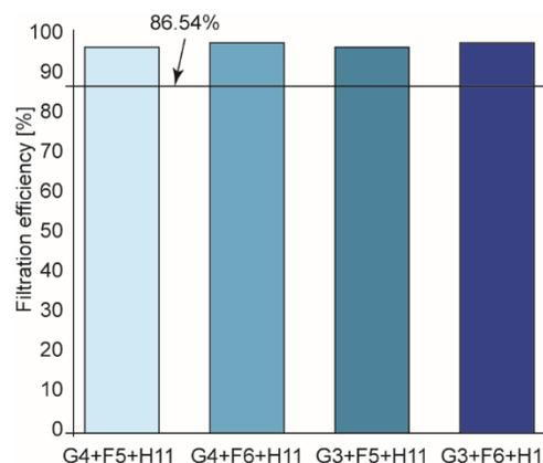
**Figure 4. The filtration efficiency of three-stage combined filters**
