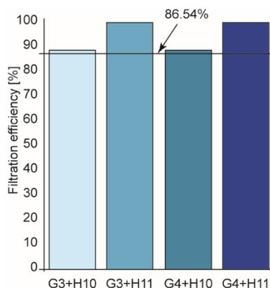
**Figure 3. The filtration efficiency of two-stage combined filters**
