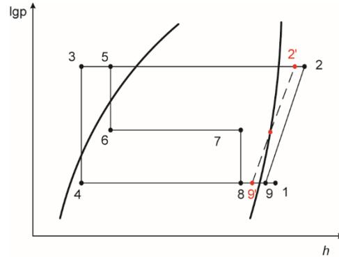
Figure 2. Cyclic pressure-enthalpy diagram of low pressure air-supply theory
