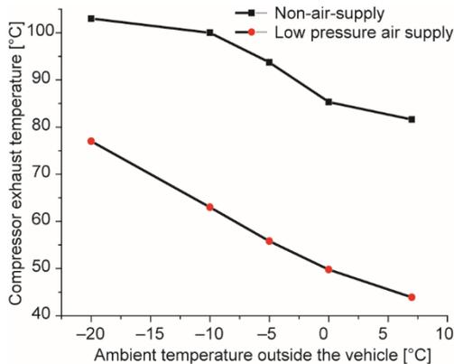
**Figure 7.** Variation of exhaust temperature of compressor with ambient temperature outside the vehicle
