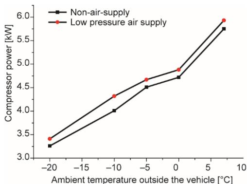
**Figure 9.** Variation of compressor power with ambient temperature outside the vehicle
