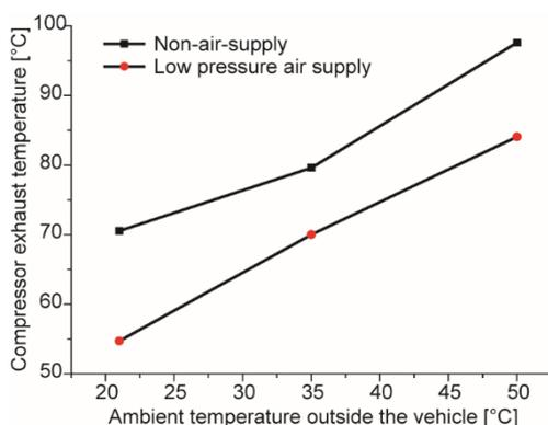
**Figure 3.** Variation of exhaust temperature of compressor with ambient temperature outside the vehicle
