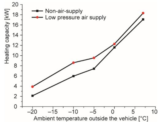
**Figure 8.** Variation of heating capacity of system with the ambient temperature outside the vehicle
