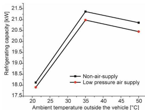
**Figure 4.** Variation of refrigerating capacity of the system with ambient temperature outside the vehicle
