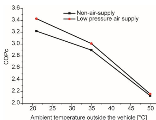
**Figure 6. Variation of system COP<sub>c</sub> with ambient temperature outside the vehicle**
