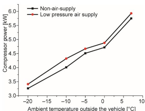
**Figure 5. Variation of compressor power with ambient temperature outside the vehicle**
