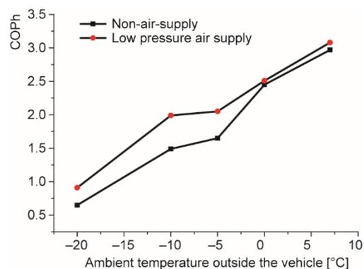
**Figure 10.** Variation of  $COP_h$  with ambient temperature outside the vehicle
