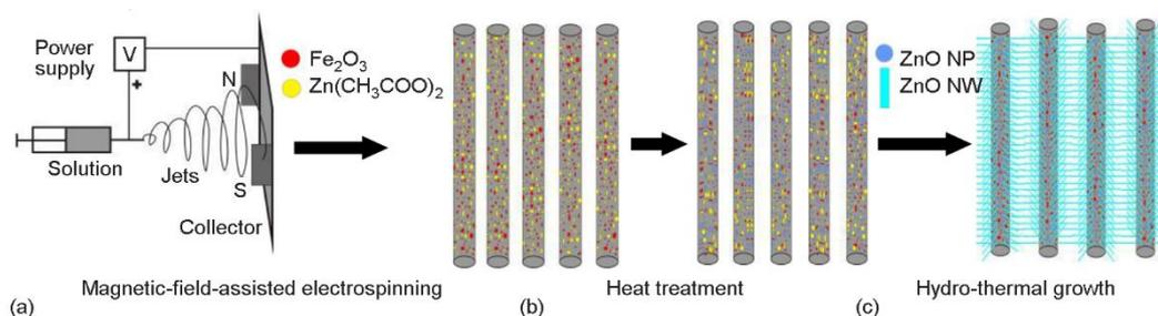
**Figure 2. Schematic illustration for the preparation process of hierarchical aligned ZnO nanorods on surface of PVDF/Fe<sub>2</sub>O<sub>3</sub> composite nanofiber membranes**
