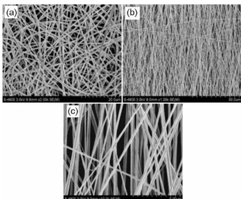
**Figure 3. The SEM images of PVDF/Fe<sub>2</sub>O<sub>3</sub>/Zn(Ac)<sub>2</sub>; (a) misaligned and (b)-(c) aligned**
