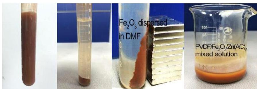
Figure 1. The Fe<sub>2</sub>O<sub>3</sub> nanoparticles dispersed in DMF solution and electrospun solutions
