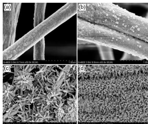
**Figure 4. The SEM images of unheated (a) and heated (b) nanofibers; (a) misaligned, (b-c) aligned, after hydro-thermally treated (c) and (d)**
