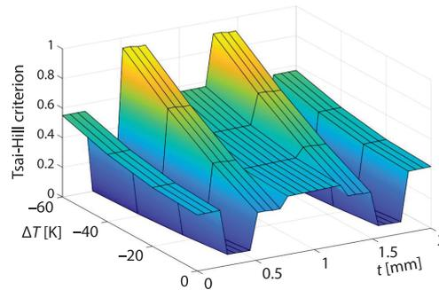
Figure 6. The mTH failure criterion values for load Case B
