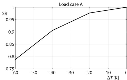
**Figure 7. Minimum SR values in the laminate for load case A**
