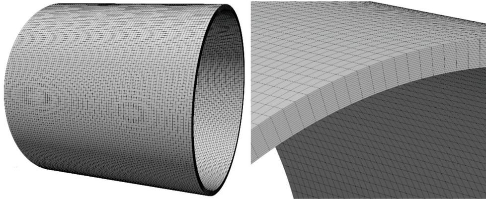
Figure 4. Finite element mesh for the cylinder analysis
