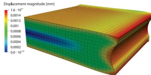
**Figure 2. Thermally loaded plate deformed shape (100 displacement scale factor, 1/4 of the model)**
