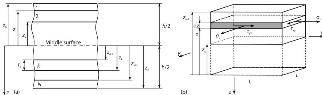
Figure 1. (a) Laminated plate geometry with numbering and (b) stresses in the  $k^{\text{th}}$  lamina
