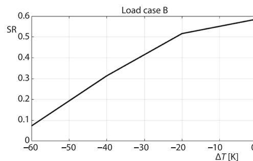
**Figure 8 – Minimum SR values in the laminate for load case B**
