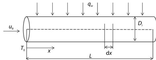
Figure 8. Convective heat transfer model
