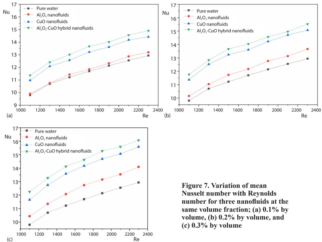
**Figure 7. Variation of mean Nusselt number with Reynolds number for three nanofluids at the same volume fraction; (a) 0.1% by volume, (b) 0.2% by volume, and (c) 0.3% by volume**
