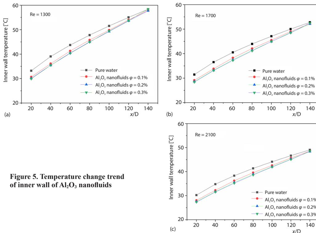
Figure 5. Temperature change trend of inner wall of  $\text{Al}_2\text{O}_3$  nanofluids
