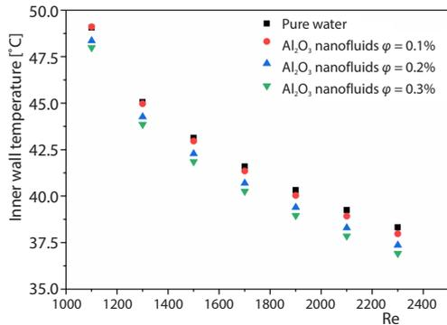
**Figure 6. Average temperature of inner wall at different Reynolds number**
