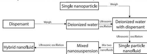
**Figure 1. Two-step preparation of hybrid nanofluids**
