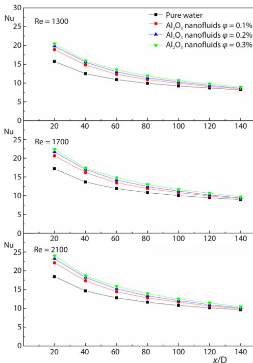
Figure 3. Change trend curve of Nu with  $x/D$  for  $\text{Al}_2\text{O}_3$  nanofluids with different volume fractions
