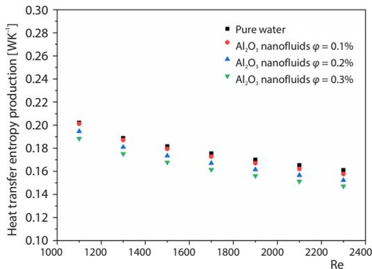
Figure 9. Change of heat transfer entropy production with Reynolds number
