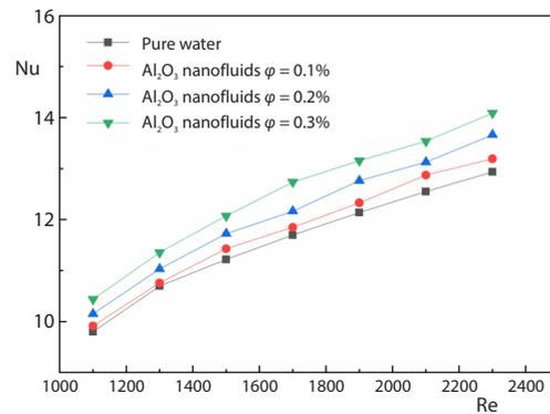
Figure 4. Average Nu of  $\text{Al}_2\text{O}_3$  nanofluids with different volume fractions vs. Reynolds number
