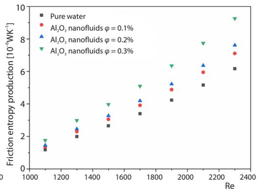
Figure 10. Change of friction entropy production with Reynolds number
