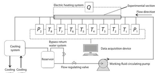
**Figure 2. Schematic diagram of the flow heat transfer experimental platform in the tube for nanofluids**
