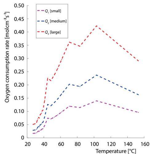
**Figure 4. Change in oxygen consumption rate for different air-leakage rates**
