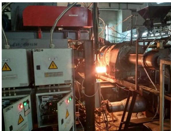
Figure 6. Photograph of an experimental set-up with a working high-voltage AC plasmatron
