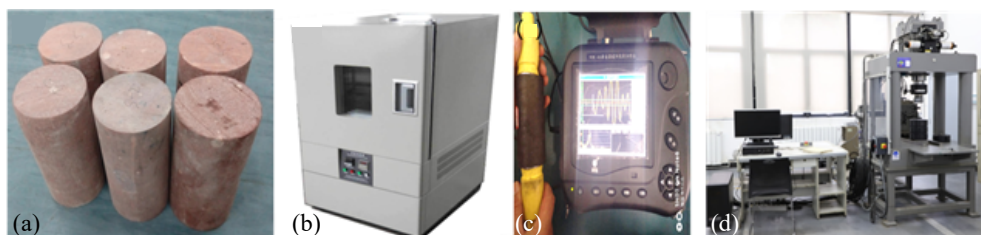
Figure 1. Sandstone samples and experimental equipments; (a) sandstone samples, (b) high temperature heating chamber, (c) NM-4A non-metal ultrasound detector, and (d) MTS-816
