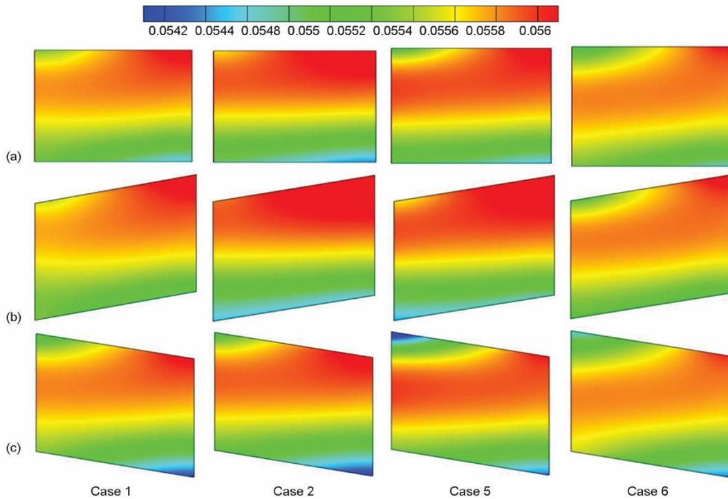
Figure 9. Comparison nanoparticle volume fraction between enclosures into (a) rectangular, (b) parallelogram with positive angle, and (c) parallelogram with negative angle
