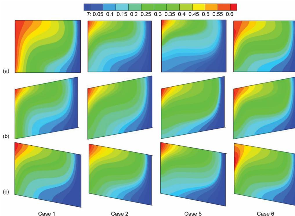
**Figure 7. Comparison temperature fields between enclosures into (a) rectangular, (b) parallelogram with positive angle, and (c) parallelogram with negative angle**
