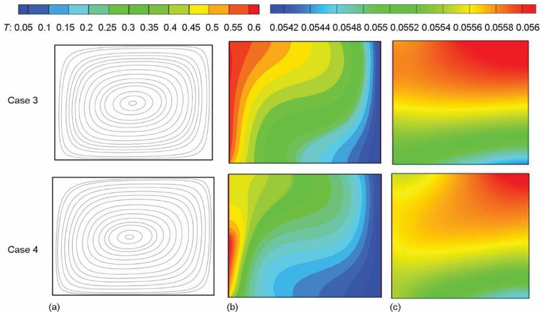
**Figure 5. Comparison streamline (a), temperature fields (b), and nanoparticle volume fraction (c) between Cases 3 and 4**
