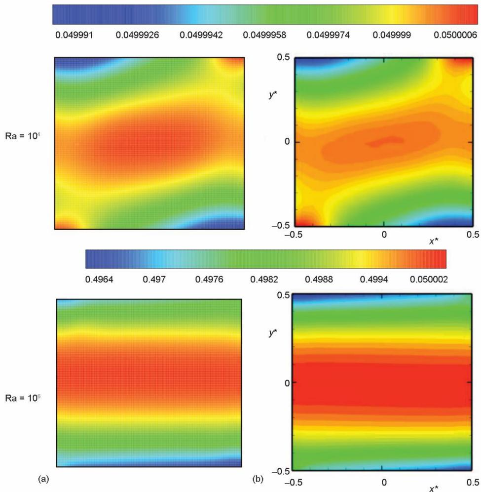
**Figure 3. Nanoparticle volume fraction distribution at  $Ra = 10^6$  in (a) present study, (b) [40]**
