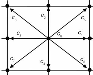
**Figure 2. The 2-D vectors for nine-velocity and temperature lattice**
