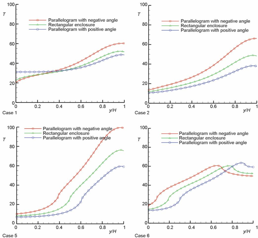
**Figure 6. Comparison temperature fields between different enclosures under different heat flux**
