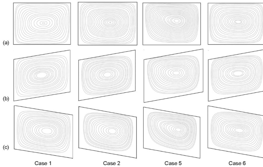
Figure 8. Comparison streamline between enclosures into (a) rectangular, (b) parallelogram with positive angle, and (c) parallelogram with negative angle
