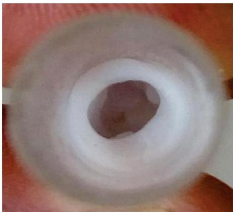
Figure 5. The PCM cavity formation inside the tube during the cooling process
