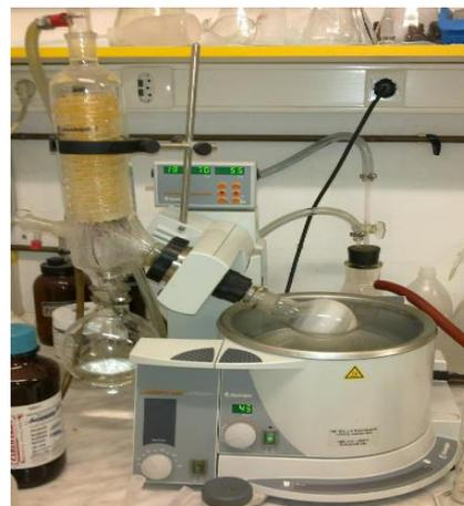
**Figure 1. Laboratory rotary evaporator (Laborota 4000 Efficient, Heidolph)**
