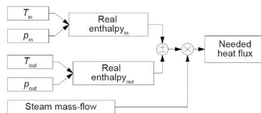
Figure 5. Schematic diagram for steam reheating between two turbines
