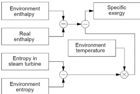
**Figure 7. Schematic diagram for the definition of the specific exergy**
