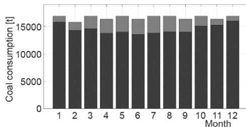
**Figure 11. Coal consumption without and with a SCRS attached to the conventional thermal power plant; light colored top of the bar marks the saved amount of coal**
