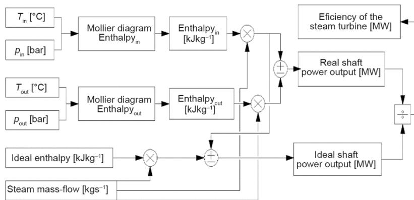
Figure 4. Schematic diagram for a high pressure steam turbine
