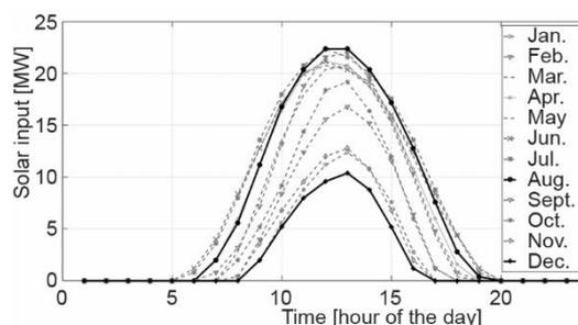
**Figure 9. Solar input of the SCRS as the function of the solar irradiance for the chosen geographical location and expected power production from the solar part of the designed model: Source of data for solar irradiation: <https://meteo.arso.gov.si/met/sl/climate>**
