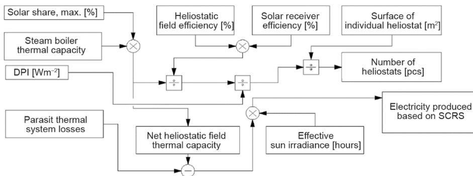
**Figure 8. The SCRS schematic diagram**
