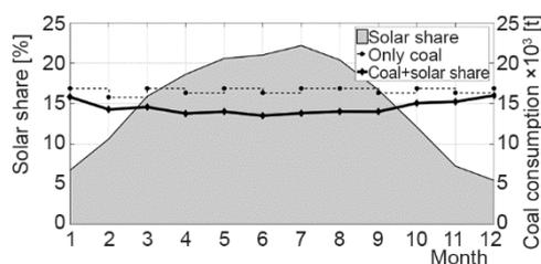
**Figure 10. Solar share vs. coal consumption for the designed analyzed model; the dotted trendline presents the reference as coal consumption of the conventional thermal power plant without a SCRS**
