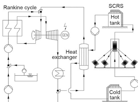
**Figure 1. Schematic presentation of combining the Rankine process with SCRS**
