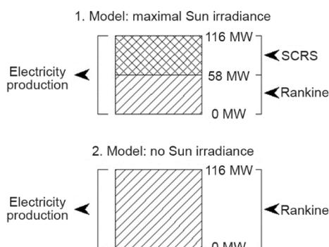
**Figure 3. Schematic presentation of two possible scenarios for the proposed model operating with maximal Sun irradiance and with no sun irradiance**
