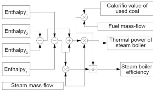
**Figure 6. Schematic diagram for the definition of steam boiler thermal power capacity and efficiency**
