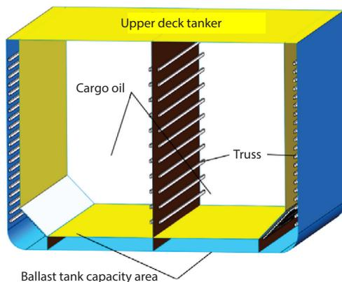
**Figure 1.** Partial schematic diagram of cargo tanks of a double hull oil tanker
