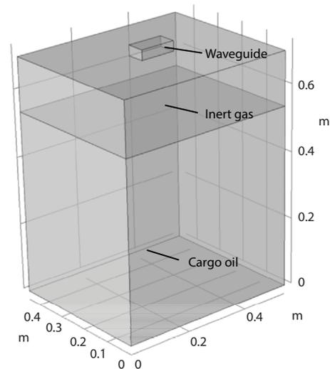
Figure 2. Schematic model of coupled electromagnetic and thermal flow of cargo oil
