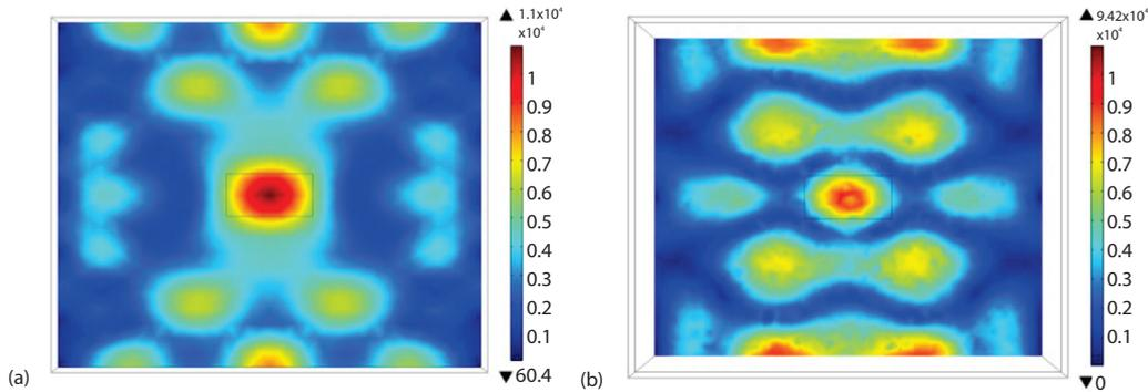
**Figure 6. Distribution of electric field strength in the heating chamber; (a)  $Z = 0.54$  m on the upper surface (b)  $Z = 0.02$  m on the bilge**
