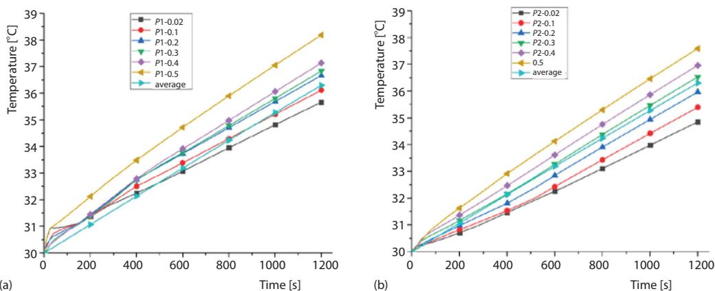
Figure 7. Time-domain changes of oil temperature at different monitoring points; P1 (a) and P2 (b) in the longitudinal direction
