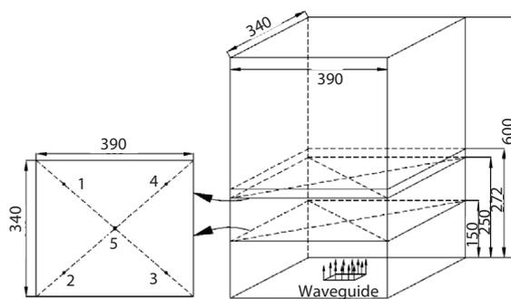
**Figure 3. Distribution of temperature monitoring points**
