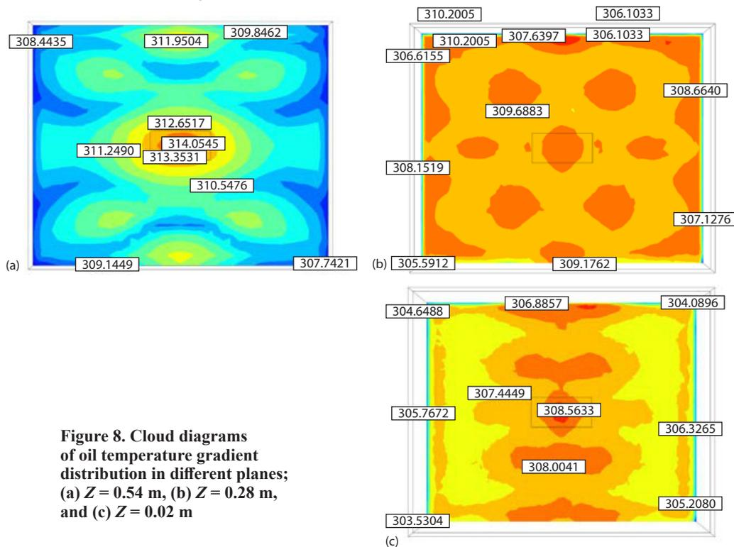
Figure 8. Cloud diagrams of oil temperature gradient distribution in different planes; (a)  $Z = 0.54$  m, (b)  $Z = 0.28$  m, and (c)  $Z = 0.02$  m
