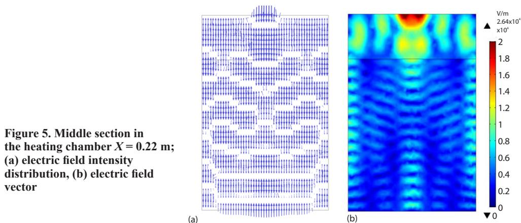
**Figure 5. Middle section in the heating chamber  $X = 0.22$  m; (a) electric field intensity distribution, (b) electric field vector**
