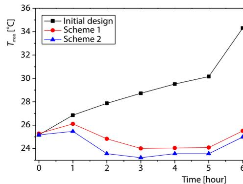
Figure 3. Maximum temperature rise curve of the set of cells with cooling structure under three different schemes
