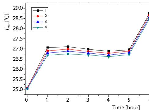
Figure 6. Variation curve of maximum temperature of each battery with time under 2C discharge rate
