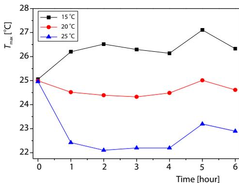
**Figure 5. Influence of different inlet temperatures of coolant on battery thermal management performance**
