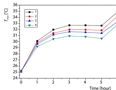
Figure 7. Variation curve of maximum temperature of each battery with time under 3C discharge rate
