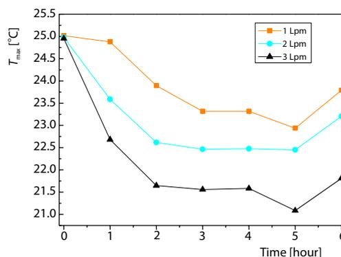
Figure 4. Influence of different coolant flows on heat dissipation performance of lithium ion battery thermal management system
