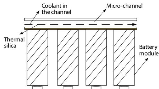
Figure 1. Design of cooling structure of set of cells
