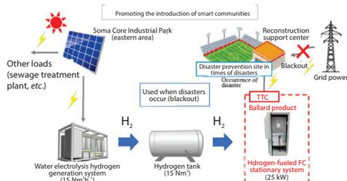
**Figure 2. Photovoltaic fuel cell cogeneration system**
