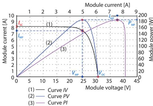
Figure 4. Characteristic curve of photovoltaic modules
