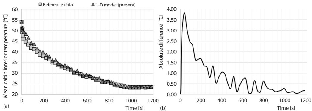
**Figure 9. (a) The comparison and (b) absolute difference of the predicted cooldown simulation results of the present and reference study**
