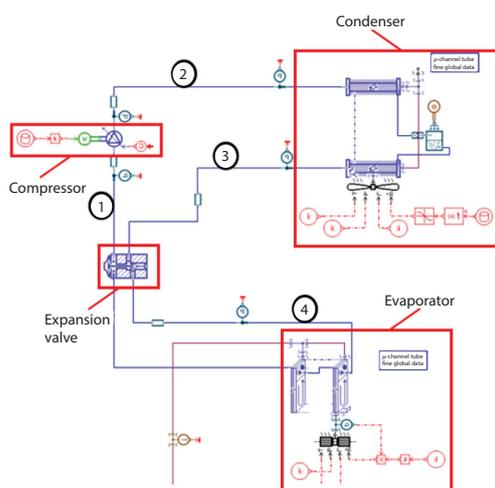
Figure 3. The Refrigerant loop 1-D model performed in this study
