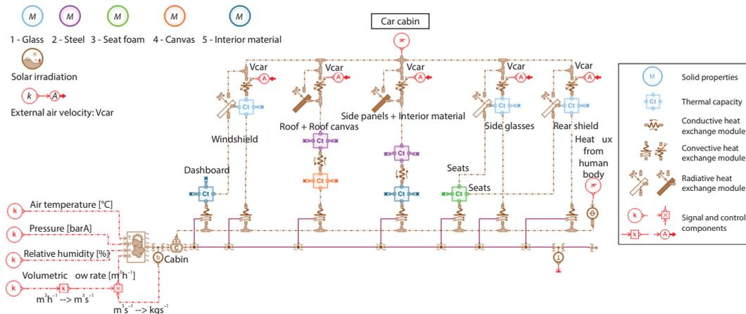
Figure 2. The developed 1-D vehicle cabin model used in soaking and cool down simulations
