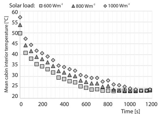
**Figure 11. Predicted mean cabin air temperature values by using R-1234yf refrigerant**
