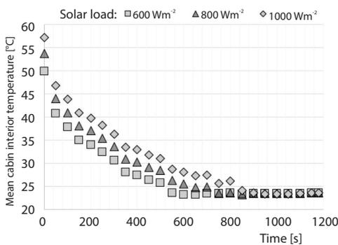
**Figure 10. Predicted mean cabin air temperature values by using R-134a refrigerant**
