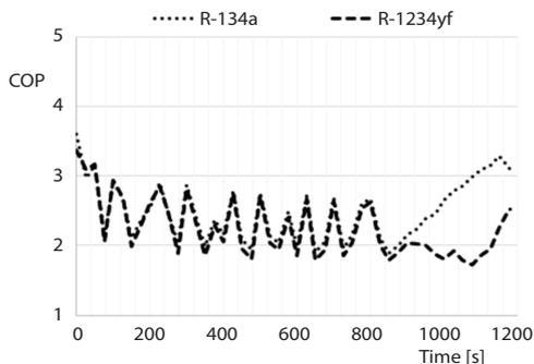
**Figure 13. The calculated COP values of the air conditioning system for 1000 W/m<sup>2</sup> solar load**
