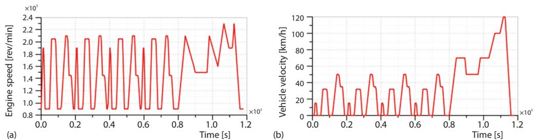
Figure 4. (a) The engine speed and (b) the NEDC driving conditions used in this study
