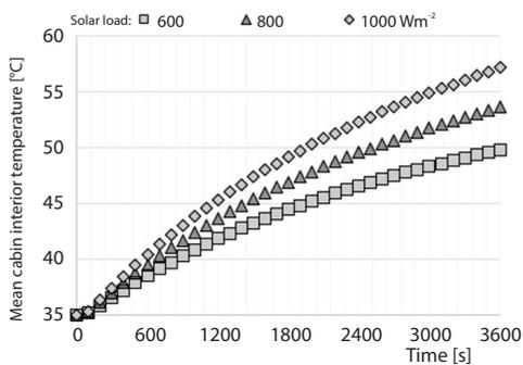
**Figure 8. The average temperature inside the vehicle cabin during the soaking period**
