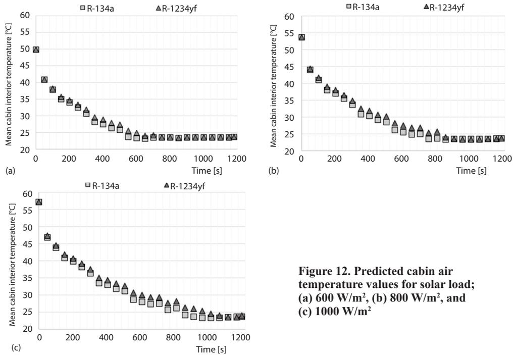
**Figure 12. Predicted cabin air temperature values for solar load; (a) 600 W/m<sup>2</sup>, (b) 800 W/m<sup>2</sup>, and (c) 1000 W/m<sup>2</sup>**
