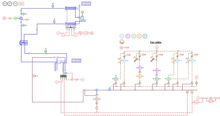
**Figure 6. The combined 1-D model include a vehicle cabin and refrigerant loop used in this study**
