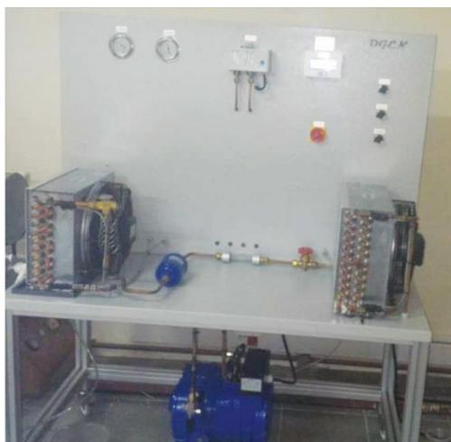
**Figure 1. Vapor-compression refrigeration system; elements: condenser, evaporator, expansion valve, pressure and temperature indicators, max-min pressure control**
