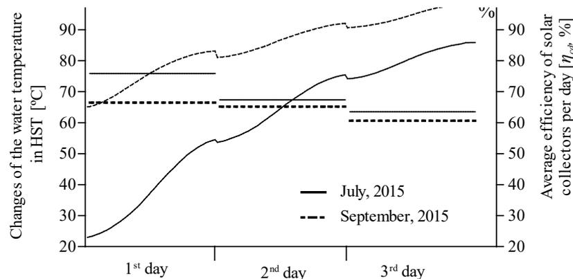
**Figure 4. Temperatures changes in HST of the three-day periods before and after curing and average efficiency of SHI**
