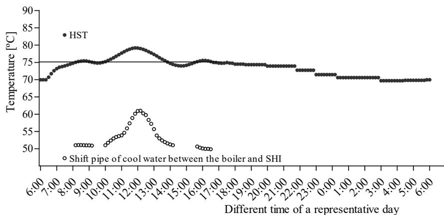
Figure 3. Daily temperature changes of water in the HST and the shift pipe of cool water
