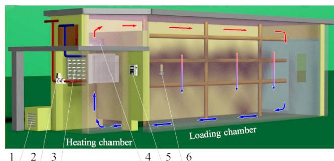
**Figure 2. Diagram of interior structure of a single bulk curing barn;** 1 – moisture-exPELLing louver for each barn, 2 – electric water-control sub-valve for each barn, 3 – heat exchanger (water-air-type), 4 – circulating fan, 5 – automatic tobacco-curing controller, 6 – sensors of dry-bulb and wet-bulb temperatures. Note: The arrow indicates the direction of the cyclic air
