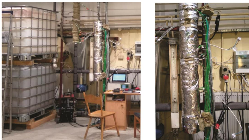
Figure 2. General view of the stand for determining the heat transfer coefficient on the inner surface of the elliptical tube and a view of the measuring section
