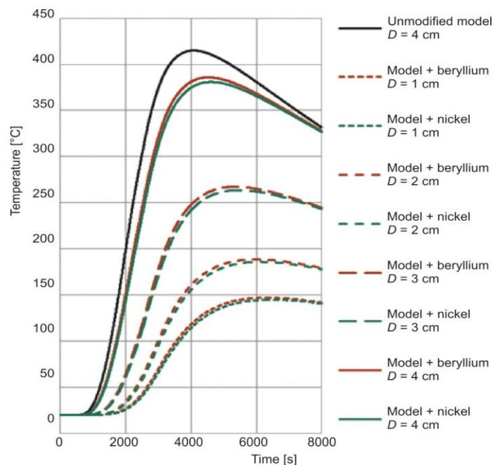
**Figure 10. Comparison of the distribution of temperature on the surface of the orbiter structure for a damaged tile with light and heavy metallic dopant,  $\gamma = 1\%$**
