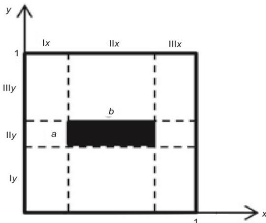
Figure 5. Location of the conductive layer inside the insulating layer in the elementary volume unit of material LI900
