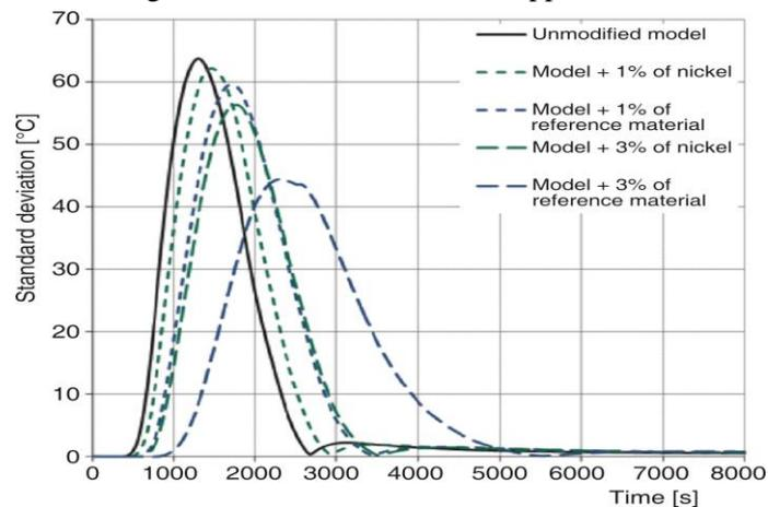
**Figure 9. Standard deviation of temperature on the surface of SIP as a function of time – damaged tile model**
