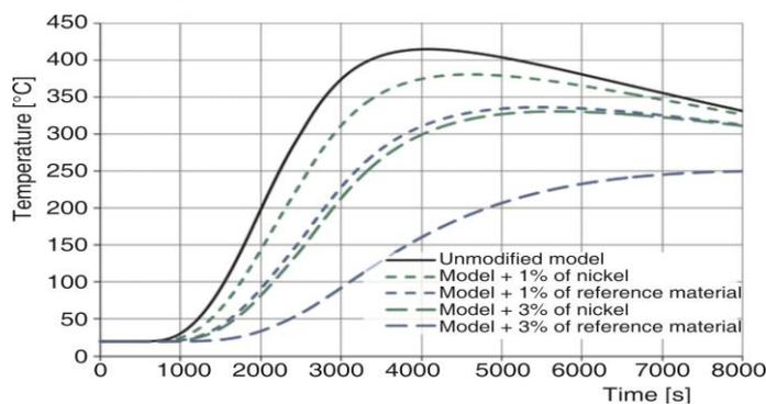
**Figure 8. Comparison of the distribution of temperature on the surface of the orbiter structure for a damaged tile**
