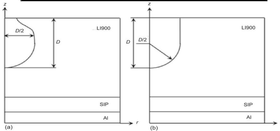
Figure 3. Geometry of damage; (a) the real model, (b) simplification
