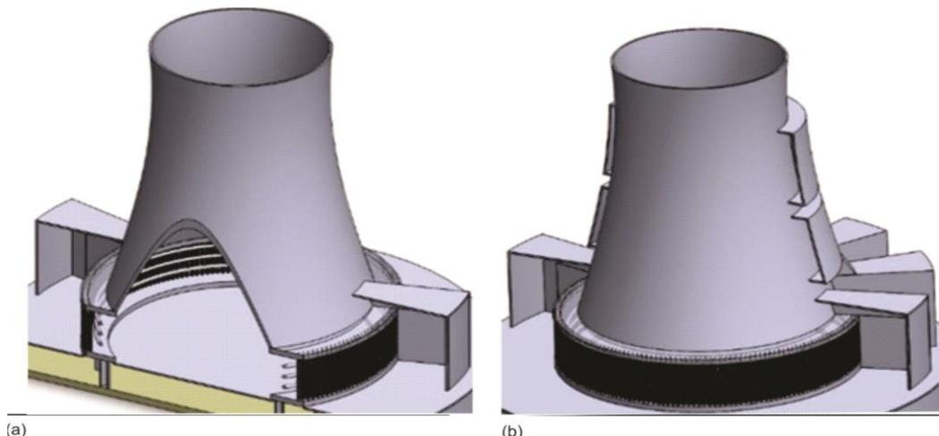
Figure 2. Experimental model of the wind collecting scheme; (a) one-duct model (b) three-duct model
