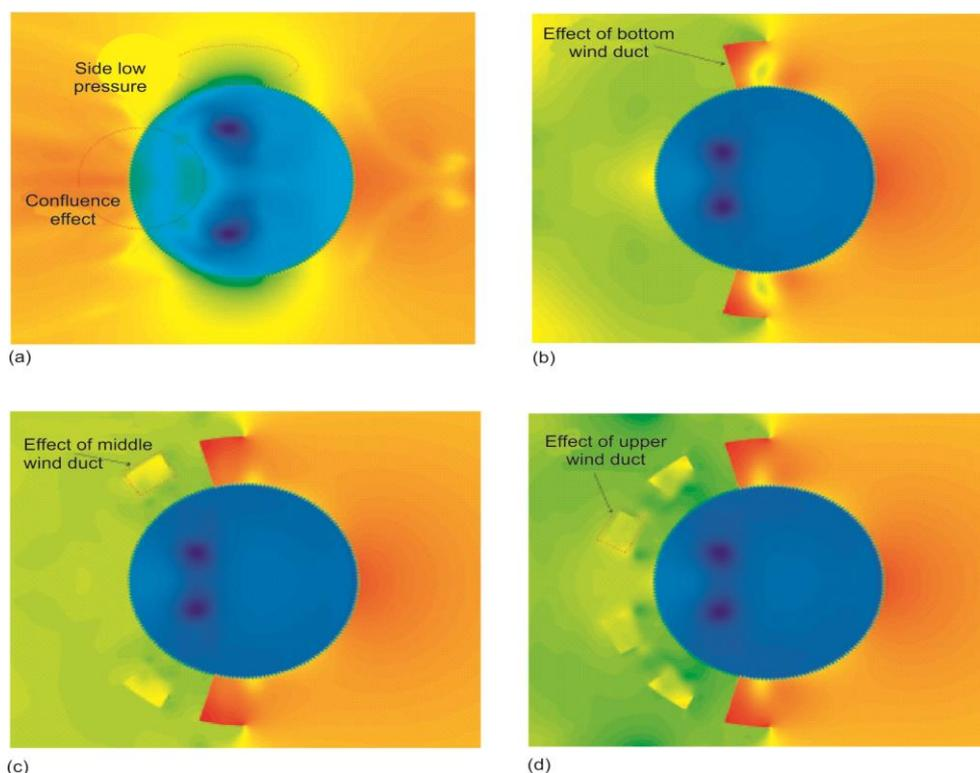
**Figure 3.** Pressure contour of the inlet middle section at 10 m/s; (a) baseline case, (b) one-duct case, (c) two-duct case, (d) three-duct case (for colour image see journal web site)
