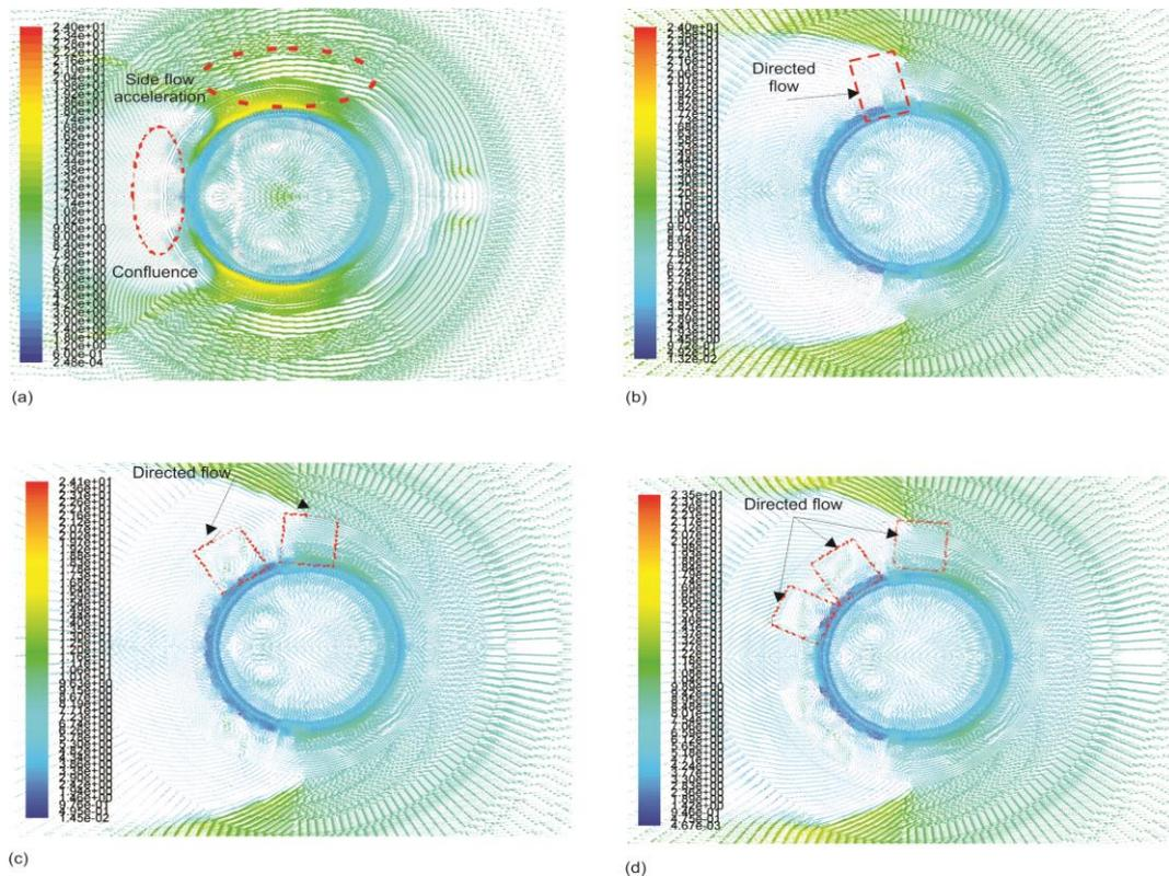
**Figure 4.** Velocity field of the inlet middle section at 10 m/s; (a) baseline case, (b) one-duct case, (c) two-duct case, (d) three-duct case (for colour image see journal web site)
