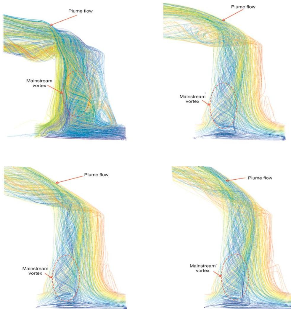
Figure 5. Streamline of the NDDCT at 10 m/s; (a) baseline case, (b) one-duct case, (c) two-duct case, (d) three-duct case (for colour image see journal web site)
