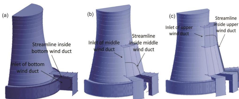
**Figure 1. Configurations of different wind collecting schemes; (a) one duct model, (b) two-duct model, (c) three-duct model**
