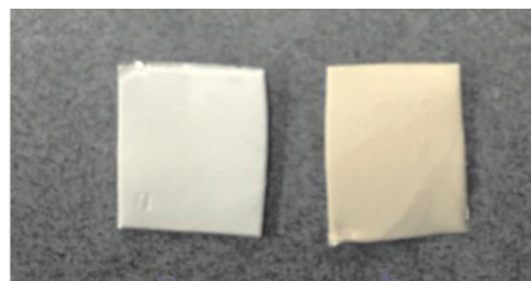
Figure 3. Nanofibers membrane; (a) PVA nanofibers membrane, (b) color rock powder-based nanofibers membrane
