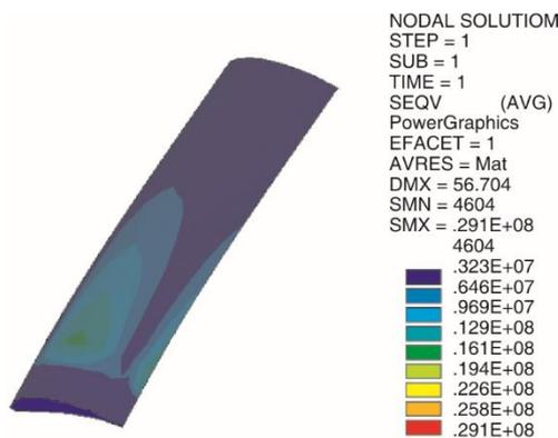
**Figure 7. Cloud image for the distribution of the overall blade stress** (for color image see journal web site)
