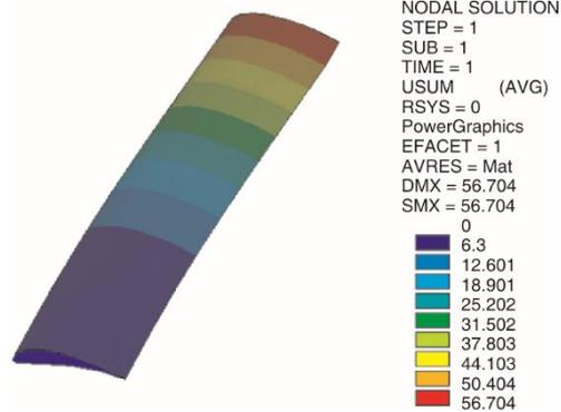
**Figure 6. Cloud image for the distribution of blade displacement** (for color image see journal web site)
