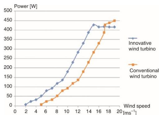
Figure 10. Performance comparison diagram for the new wind generator and the traditional unit
