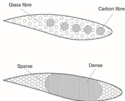
**Figure 8. Arrangement and combination of the densities of the fibers**
