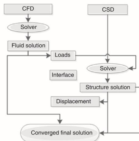
**Figure 4. The algorithm for partitioning the numerical simulation for air operated flexibility**
