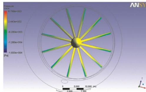
**Figure 2. Force analysis of the blade in the air-flow** (for color image see journal web site)
