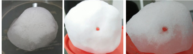
Figure 1. Snow sample. A rod with high temperature was inserted into the center of the snow
