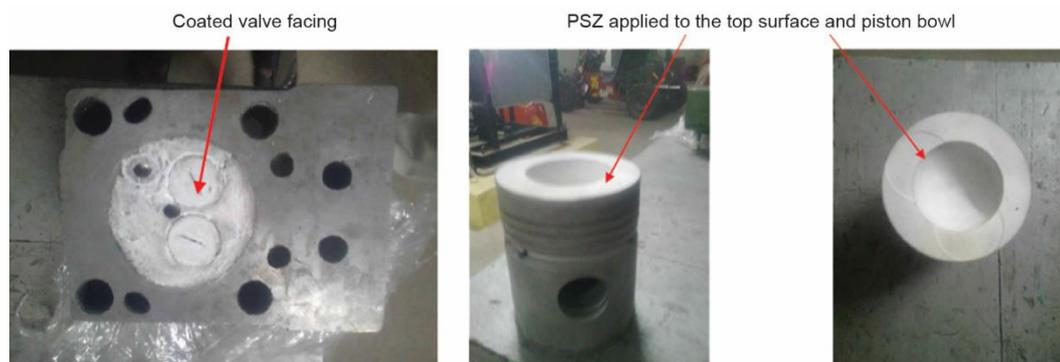
Figure 1. Photographic view of cylinder head and piston bowl
