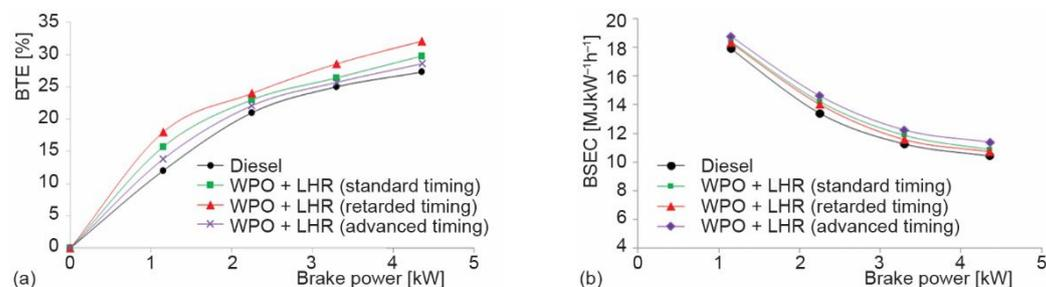
Figure 3. (a) The BTE vs. brake power, (b) BSEC vs. brake power
