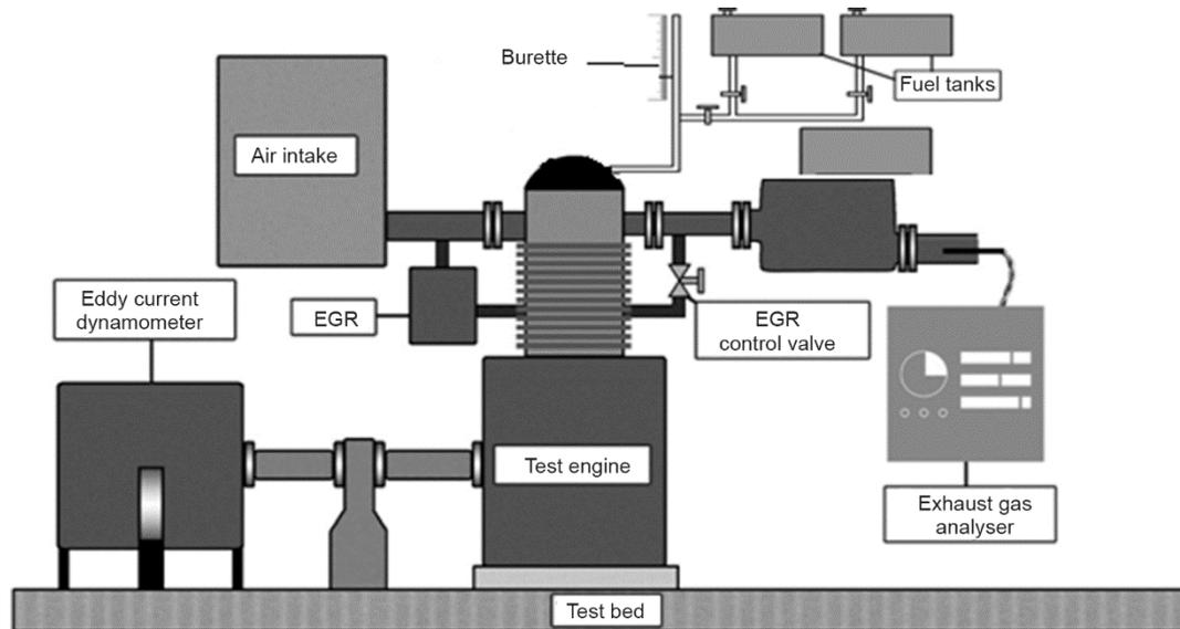
Figure 2. Schematic layout of the variable compression ratio (VCR) engine
