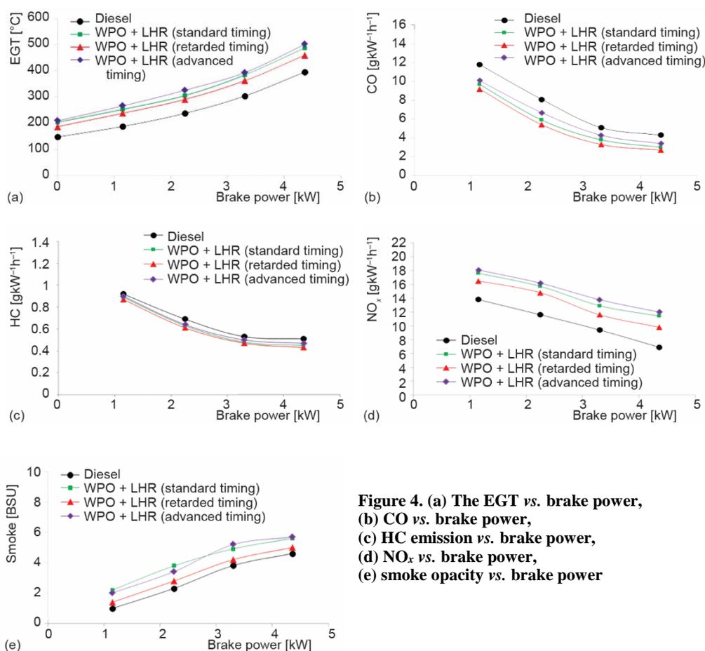
**Figure 4. (a) The EGT vs. brake power, (b) CO vs. brake power, (c) HC emission vs. brake power, (d) NO<sub>x</sub> vs. brake power, (e) smoke opacity vs. brake power**
