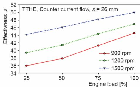
**Figure 5. Effectiveness vs. engine load for different engine speed**
