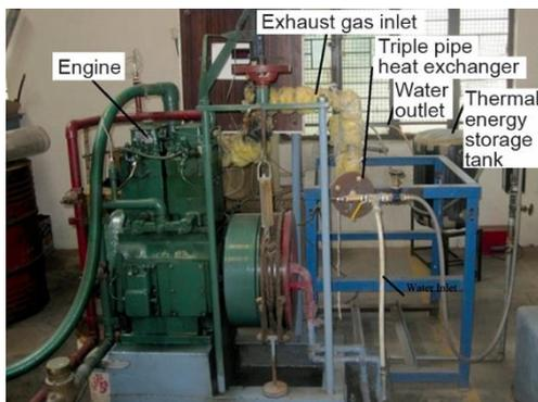
Figure 1. Experimental set-up pictorial view
