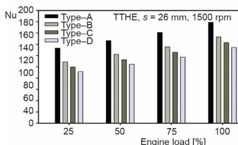
Figure 3. Variation of Nusselt numbers vs. different flow pattern of TTHE
