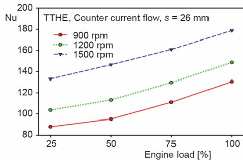
**Figure 6. Nusselt number vs. engine load for different engine speed**
