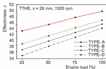
Figure 4. Variation of Effectiveness vs. different flow pattern of TTHE
