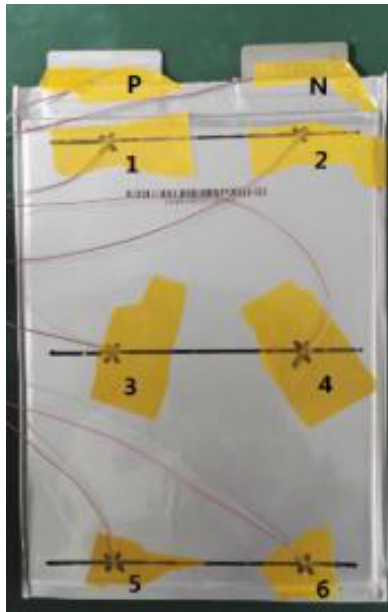
Figure 4. Lithium-ion batteries for laboratory use and their hot spot test lines
