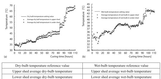
Figure 1. Distribution curves of average dry-bulb temperature; (a) and wet-bulb temperature, (b) between the upper and lower sheds in the curing barns
