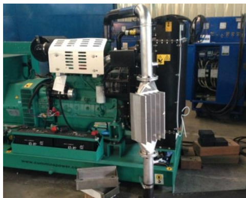
Figure 8. Diesel engine and installed positions of the TEG system
