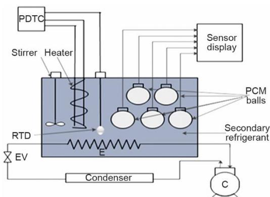
**Figure 1. Schematic diagram of the test set-up:**
