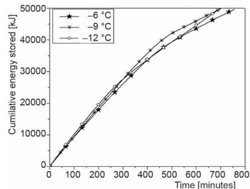
**Figure 7.** Cumulative energy stored in the storage tank for various bath temperatures (mass-flow rate  $\dot{m} = 440\text{ Lph}$ )
