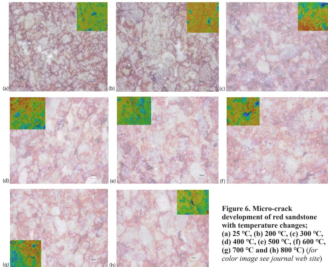
**Figure 6. Micro-crack development of red sandstone with temperature changes; (a) 25 °C, (b) 200 °C, (c) 300 °C, (d) 400 °C, (e) 500 °C, (f) 600 °C, (g) 700 °C and (h) 800 °C (for color image see journal web site)**
