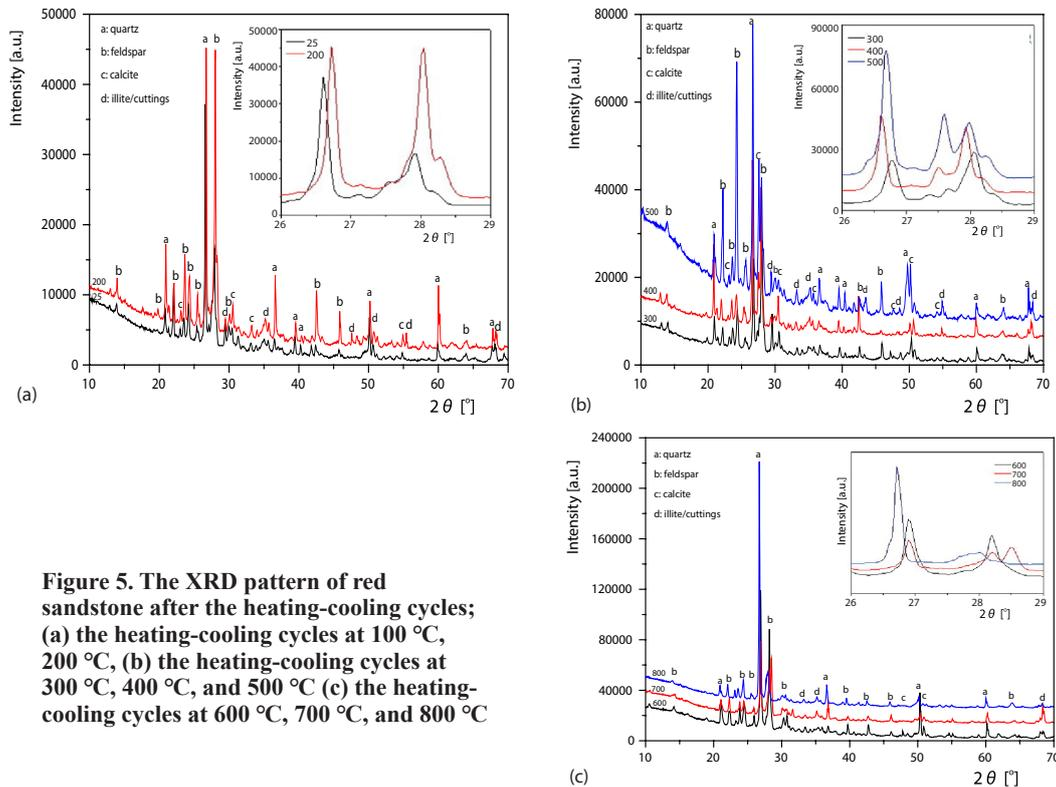
**Figure 5.** The XRD pattern of red sandstone after the heating-cooling cycles; (a) the heating-cooling cycles at 100 °C, 200 °C, (b) the heating-cooling cycles at 300 °C, 400 °C, and 500 °C (c) the heating-cooling cycles at 600 °C, 700 °C, and 800 °C
