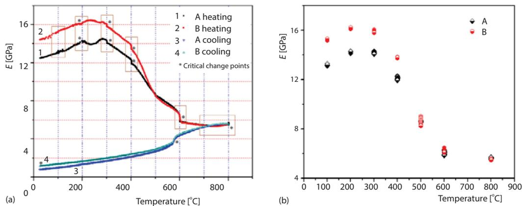
**Figure 3. (a) Variations of Young's modulus with temperature for the heating-cooling cycles, (b) Variations of Young's modulus at different gradient temperature heated on for 5 minutes**
