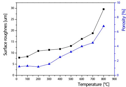
Figure 7. surface roughness of red sandstone with temperature changes
