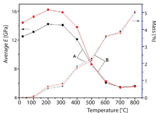
**Figure 4. The average values of Young's modulus at different temperature and mass loss of red sandstone after the heating-cooling cycles (A and B is specimen A and B)**
