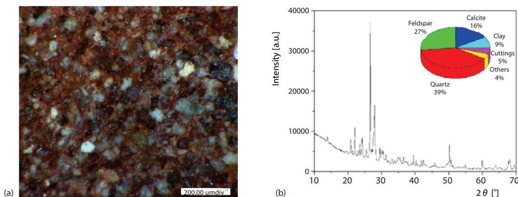
Figure 2. (a) the microscopic morphology, (b) the XRD pattern and mineral component of red sandstone at room temperature
