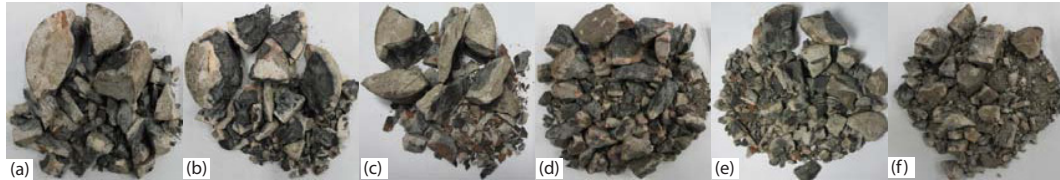
Figure 7. The tensile failure of sandstone specimens under different strain rate; (a) \dot{\epsilon} = 35.747 \text{ s}^{-1} , (b) \dot{\epsilon} = 39.179 \text{ s}^{-1} , (c) \dot{\epsilon} = 60.255 \text{ s}^{-1} , (d) \dot{\epsilon} = 69.412 \text{ s}^{-1} , (e) \dot{\epsilon} = 72.125 \text{ s}^{-1} , and (f) \dot{\epsilon} = 77.888 \text{ s}^{-1}
