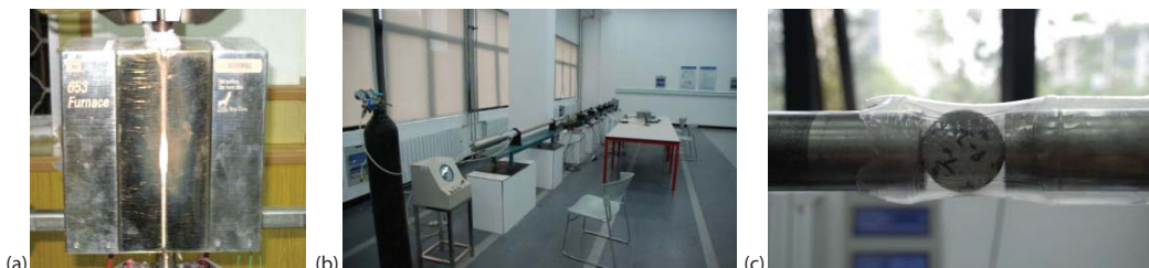
Figure 1. Test equipment and sample loading method; (a) the MTS652.02 high temperature furnace, (b) the SHPB test system, and (c) sample loading method
