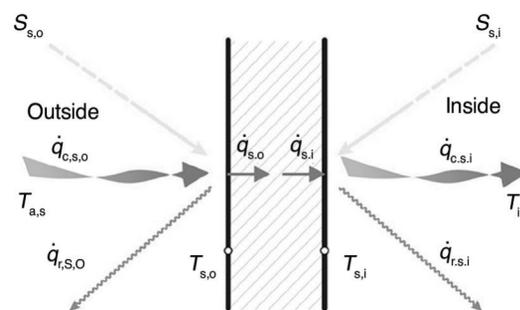
Figure 2. Surface heat fluxes and temperatures [14]
