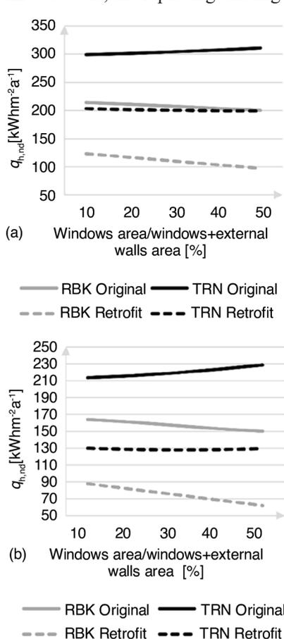
**Figure 3. Heating energy needed for theoretical; (a) single-story house with square base and (b) two-story house with square base**
