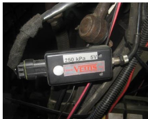
Figure 7. The MAP sensor mounted on the engine [23]
