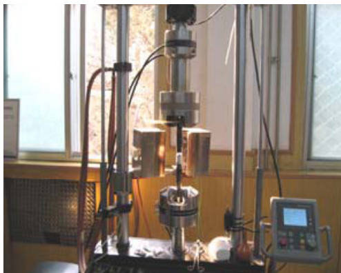
Figure 1. Matching of MTS810 and MTS652.02
