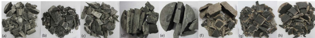
Figure 4. Sandstone failure morphology at different temperatures; (a) 25 °C, (b) 100 °C, (c) 200 °C, (d) 400 °C, (e) 500 °C, (f) 600 °C, (g) 700 °C, and (h) 800 °C
