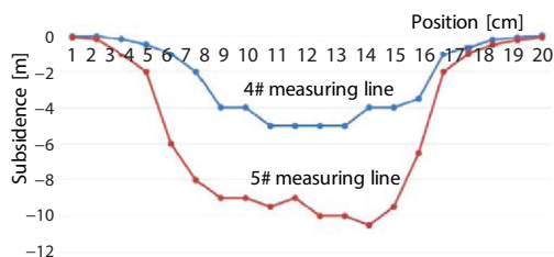
Figure 5. Roof subsidence curve
