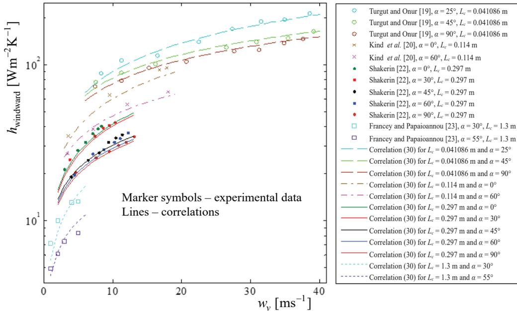
**Figure 2.** Comparisons of correlations (29) and (30) with heat transfer coefficients due to forced convection calculated from the existing experimental data (*for color image see journal web site*)
