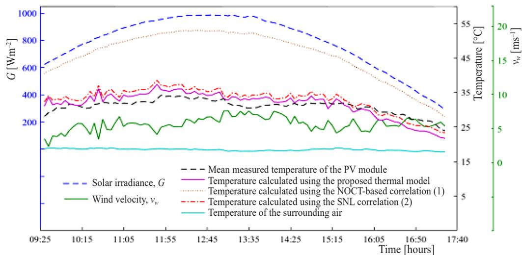
**Figure 5. Comparison between measured and calculated temperatures of the mono-crystalline PV module when it is inclined at an angle of  $37^\circ$  to the horizontal for different values of  $T_a$ ,  $v_w$ , and  $G$  [29] (for color image see journal web site)**
