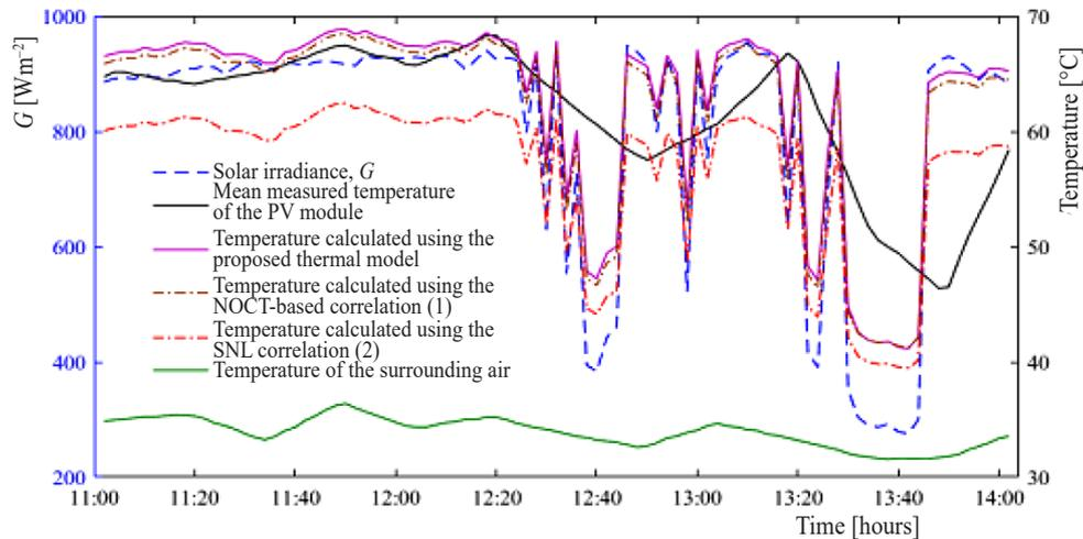
**Figure 6. Comparison between measured and calculated temperatures of the mono-crystalline PV module which is positioned horizontally and analysed in [30] for different values of  $T_a$  and  $G$  (for color image see journal web site)**
