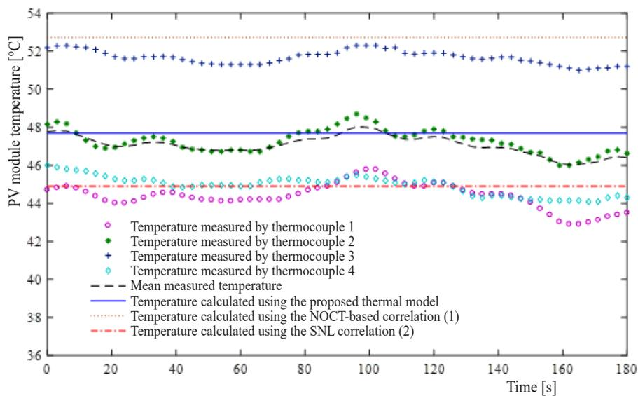
**Figure 4. Comparison between measured and calculated temperatures of the poly-crystalline PV module of the type SL-50P when it is inclined at an angle of 20° to the horizontal (for color image see journal web site)**
