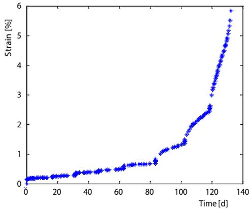
Figure 4. The whole-process creep curve
