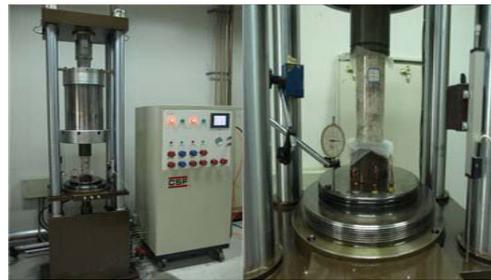
Figure 3. Experimental set-up of creep test of salt rock
