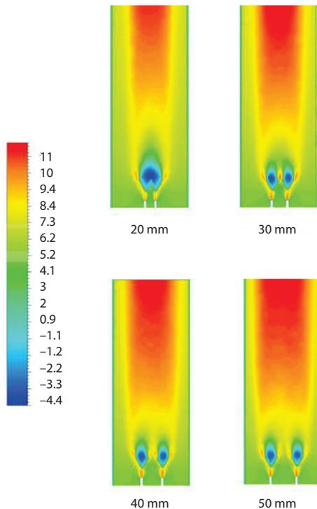
**Figure 10. Numerical results of temperature fields for different distances between V-gutters at the inlet velocity of 5 m/s**
