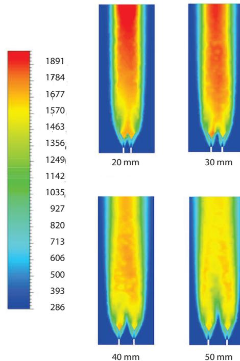
Figure 9. Numerical results of temperature fields for different distances between V-gutters at an inlet velocity of 5 m/s
