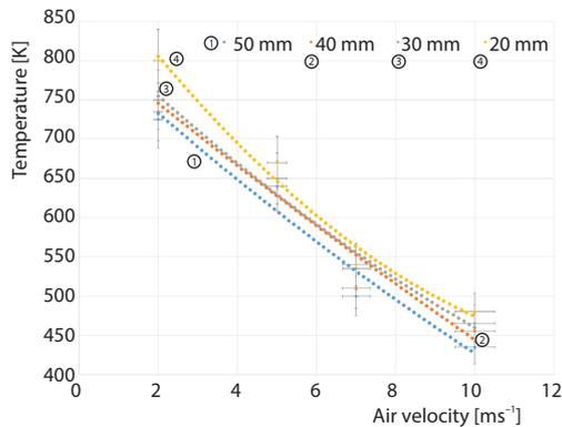
**Figure 6.** Influence of distance between V-gutters on exhaust gas temperature
