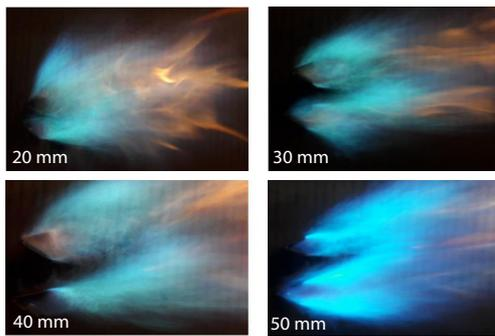
**Figure 7.** Flame photos for different distances between V-gutters at the same velocity of 5 m/s
