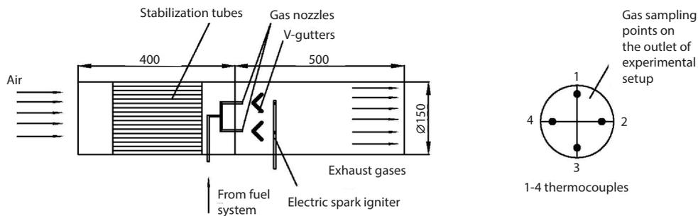
Figure 1. Schematic diagram of the combustor with a bluff body (top view)
