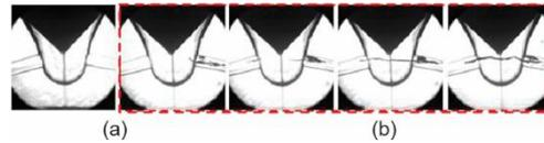
Figure 10. The geometry-induced cavitation caused by string cavitation ( $P_{in} = 1.0$  MPa,  $h = 0.5$  mm); (a) no geometry-induced cavitation and string cavitation, (b) geometry-induced cavitation appeared with the string cavitation
