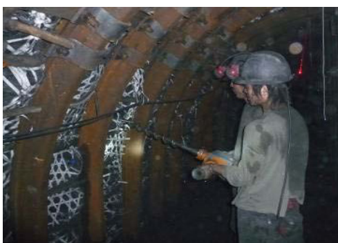
Figure 14. Miners drilling the pressure-relief hol
