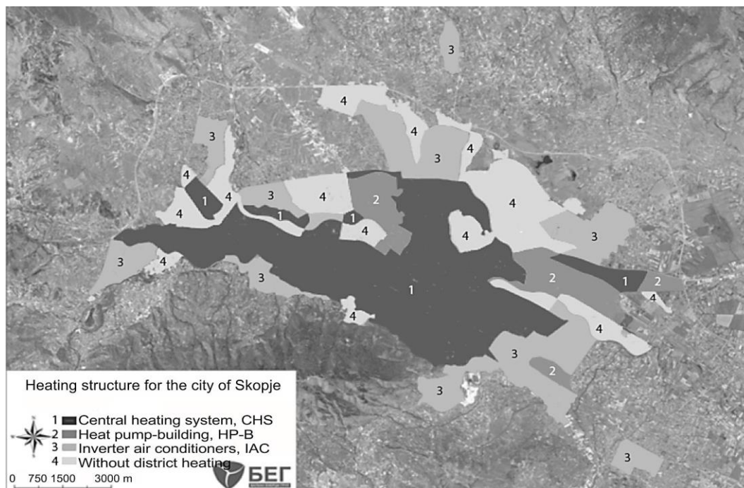
Figure 9. Techno-economic optimal heating structure for the city of Skopje (color legend, accordingly the colors in tab. 2)
