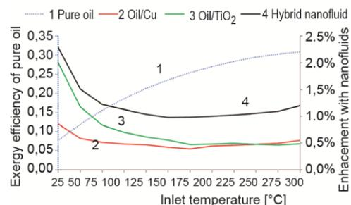
**Figure 7. Exergy efficiency results for the examined cases and inlet temperature levels between 25 °C and 300 °C**
