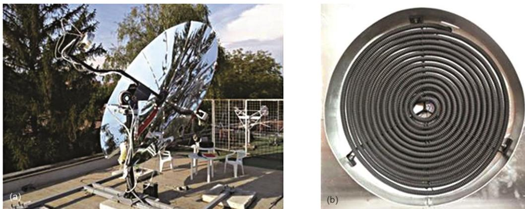
Figure 1. The experimental set-up of the solar dish collector; (a) the total collector, (b) the examined absorber
