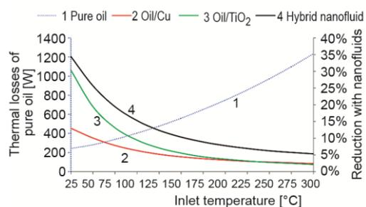
**Figure 5.** Thermal losses results for the examined cases and inlet temperature levels between 25 °C and 300 °C
