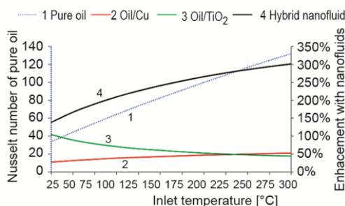
**Figure 2.** Nusselt number results for the examined cases and inlet temperature levels between 25 °C and 300 °C
