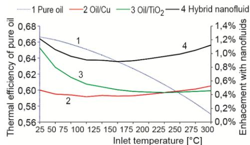
**Figure 6. Thermal efficiency results for the examined cases and inlet temperature levels between 25 °C and 300 °C**
