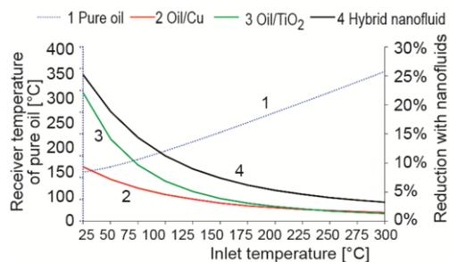
**Figure 4.** Receiver temperature results for the examined cases and inlet temperature levels between 25 °C and 300 °C
