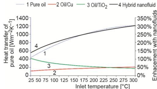
**Figure 3.** Heat transfer coefficient results for the examined cases and inlet temperature levels between 25 °C and 300 °C
