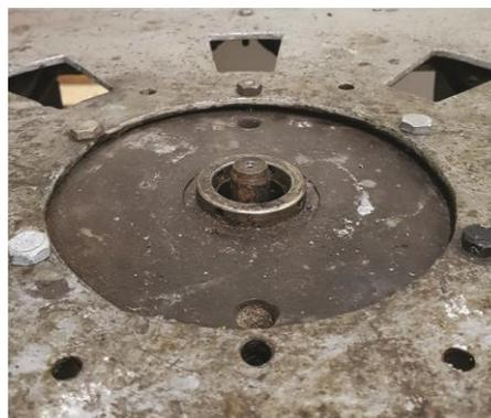
Figure 4. The diffusive combustion burner
