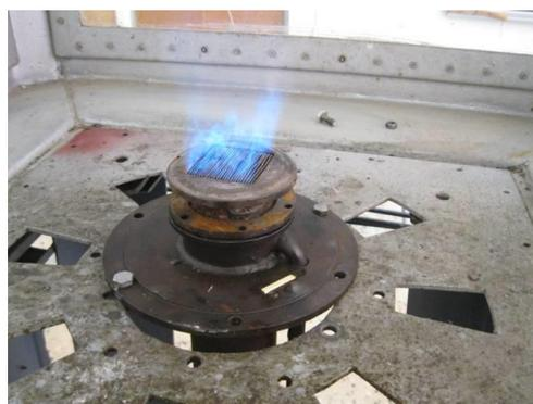
Figure 6. Flame of the stabilizer with slots burner
