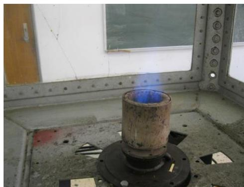
**Figure 9.** Flame aspect when using the ceramic stabilizer
