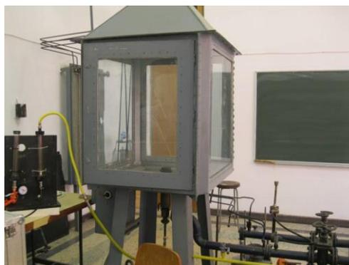
Figure 2. Experimental stand equipped with a self-aspiration burner
