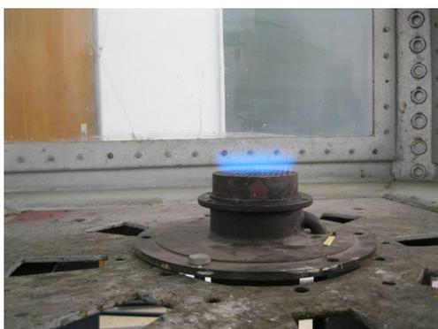
Figure 5. Flame of the stabilizer with holes
