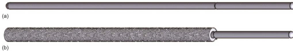
Figure 1. The 3-D models of the studied thermosyphons; (a) thermosyphon with smooth walls, (b) thermosyphon with finned tubes
