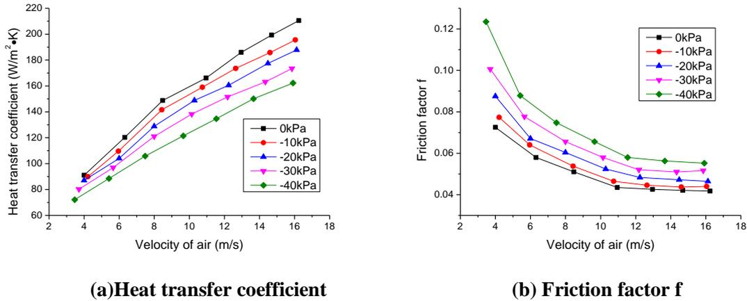
**Figure 2. Experimental results under different gauge pressure conditions**
