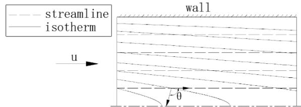
**Figure 5. Diagram of the field synergy angle (FSA)**
