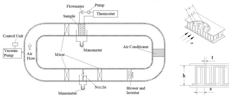
**Figure 1. Schematic diagram of the wind tunnel test apparatus and offset fin structure size**
