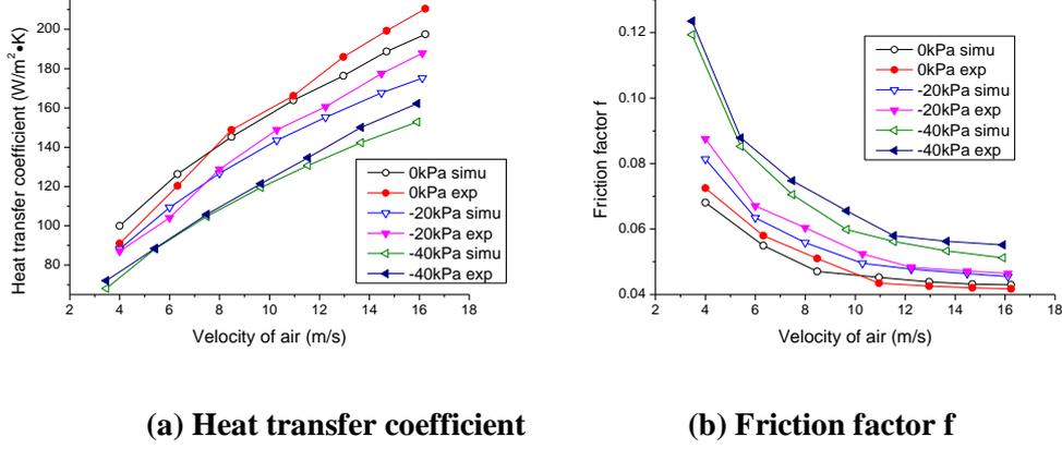
**Figure 4. Comparison of numerical results and experimental data**
