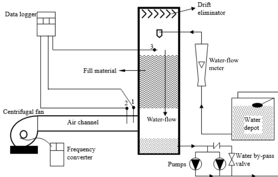
Figure 1. Schematic diagram of the experimental set-up
