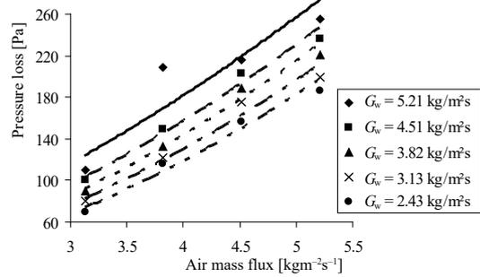
Figure 8. Pressure loss values obtained with curler type fill for 0.8 m fill height
