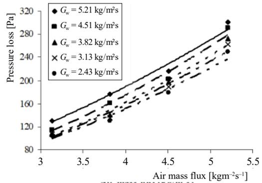
Figure 6. Pressure loss values obtained with film type fill for 1 m fill height
