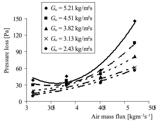
Figure 10. Pressure loss values obtained with splash type fill for 0.6 m fill height
