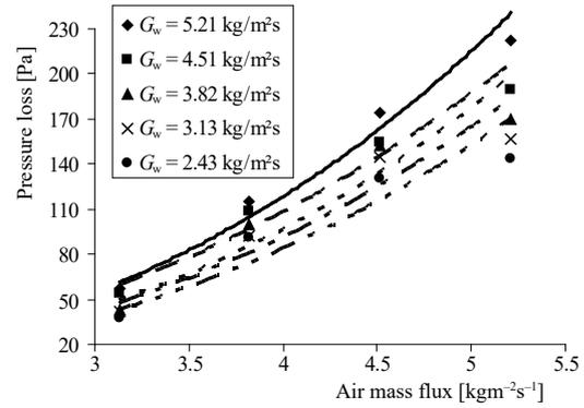
Figure 4. Pressure loss values obtained with film type fill for 0.6 m fill height
