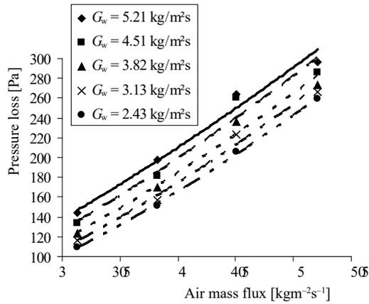
Figure 9. Pressure loss values obtained with curler type fill for 1 m fill height
