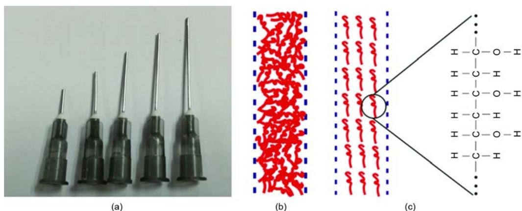
**Figure 1.** Tube samples (a) and chain distribution of PVA solution in the tube, (b) amorphous chains in a short tube, and (c) periodic chains in a long tube
