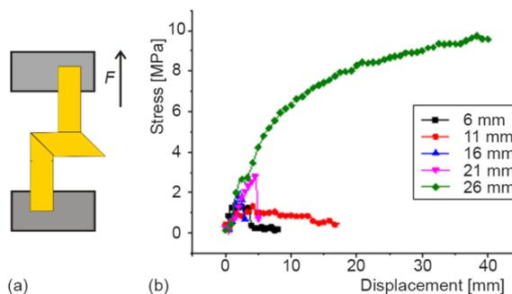
**Figure 2. Tearing process (a) and the stress-strain relationship for different tube lengths from 6 mm to 26 mm (b) (for color image see journal web site)**
