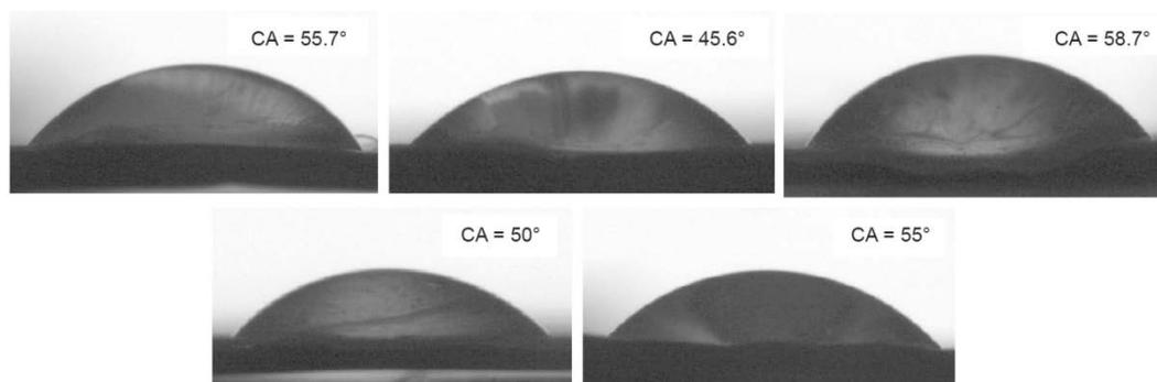
Figure 4. Wetting property of each sample with different tube lengths from 6mm to 26 mm
